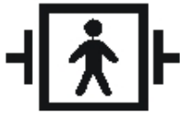
Model BF device with function for protection of electricity discharge effect from cardiac defibrillator
