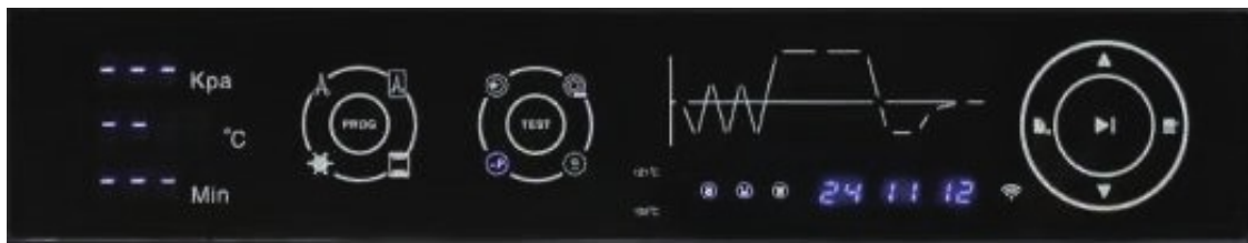
Control panel: pressure (kPa), temperature (°C) and time (min) readouts on the left, program and test function keys with the cycle curve and the date/time display in the center, navigation and start keys on the right
