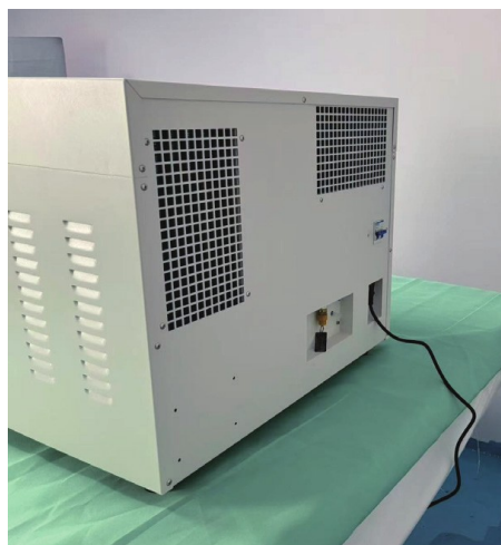
Rear side of the unit: ventilation grille, power inlet and cable outlet
